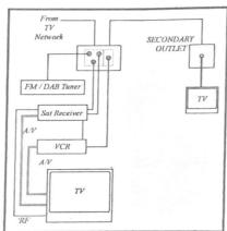
The diagram on the left illustrates the basic connections required to send TV signals to a TV in the lounge and a TV in a bedroom. The necessary connecting leads and splitter unit can be purchased from any TV dealer or by mail order from Trac Communications on 01642 712481.
